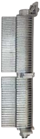
The blocking for spring hangers and spring supports types 21, 25, 29 and 20 consist of sheet metal lamellas adjustable to any desired load position. Up to 3 blocking devices can be inserted into a spring hanger.
