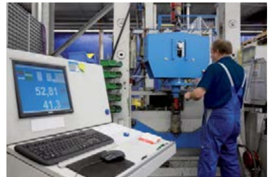
Acceptance testing of a constant hanger
