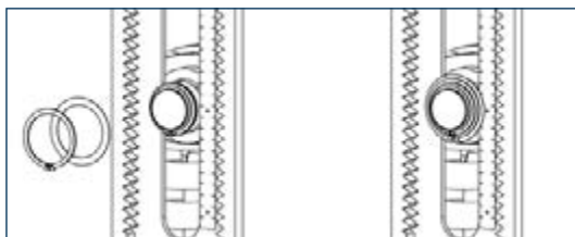
② Assembly of the outer lock ring ③ Completed: deblocked condition
