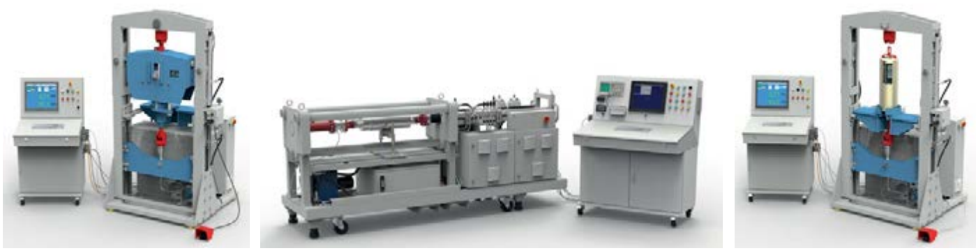
Testing a constant hanger on a LISEGA 120kN test bench
