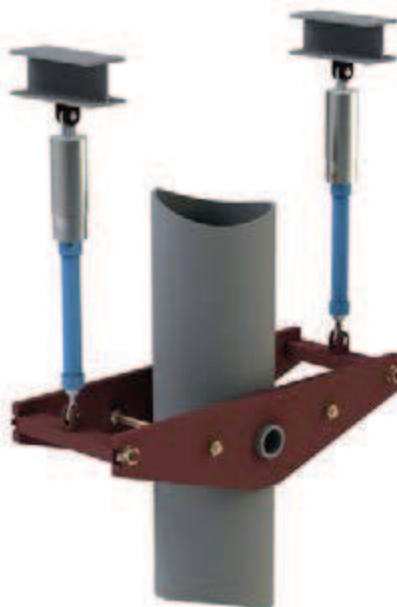
Support of a vertical pipe system section by type 30 snubbers with extension type 33 and dynamic clamp type 34.
