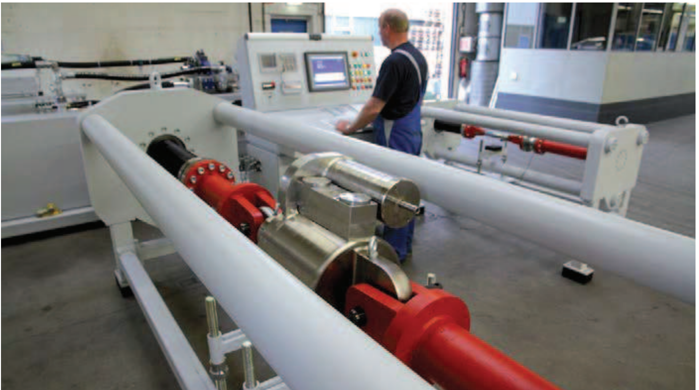
Test bench for snubbers
